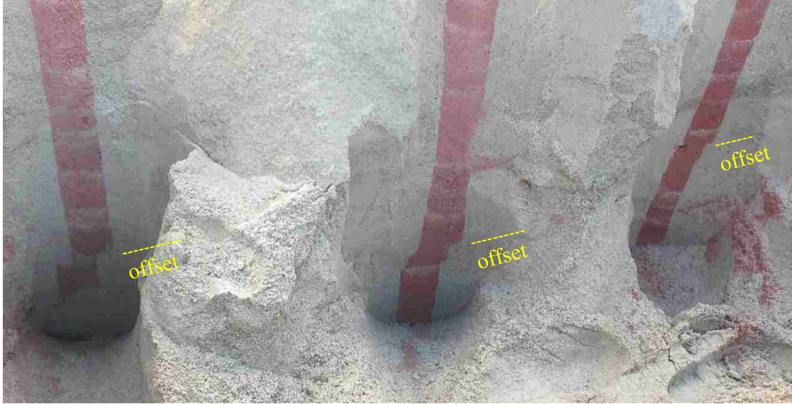
Figure 4-8: Offset in red sand columns showing the failure surface of the 30° skew test
