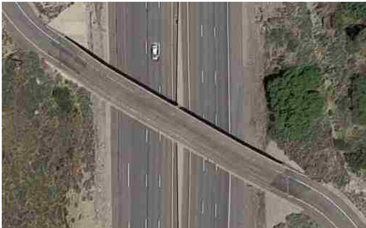
Figure 2-15: A narrow skewed bridge located near utility exit 133 off of Interstate-80, about 5 miles east of Salt Lake City, Utah (adapted from Google Earth)
