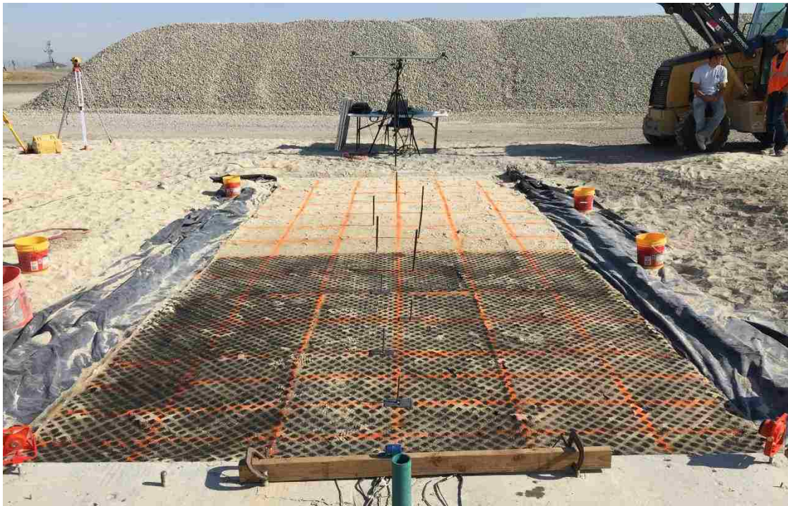
Figure 3-10: Uniform pattern of black dots painted on first 12 feet of backfill to aid the DIC camera system in tracking ground surface displacement
